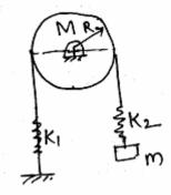
Determine the natural frequency of vibration for the system shown. Assume there is no slip between the cord and cylinder. [16]
