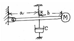
Derive the equation of motion for the system above and determine the damping coefficient under critical damping. [6+10]
