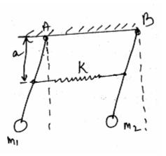
Consider two pendulums of length L shown. Determine the natural frequency of vibration for the given data K = 100 N/m,  $m_1 = 2 kg$ ,  $m_2 = 5 kg$ , L = 0.2 m, a = 0.1m. [16]
