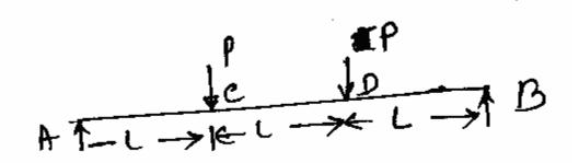
Determine the natural frequency of vibration for the above system using Dunkerley's method. [6+10]
